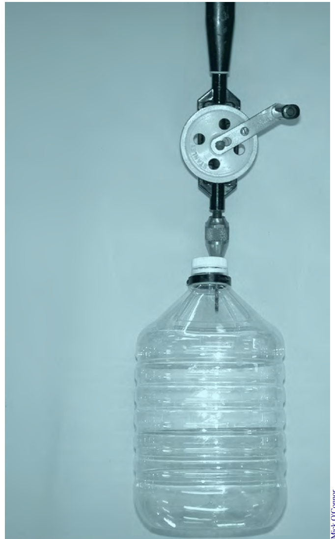
Figure 11.2 Step 1: Hold the bottle securely and drill three 3 mm holes in the cap
