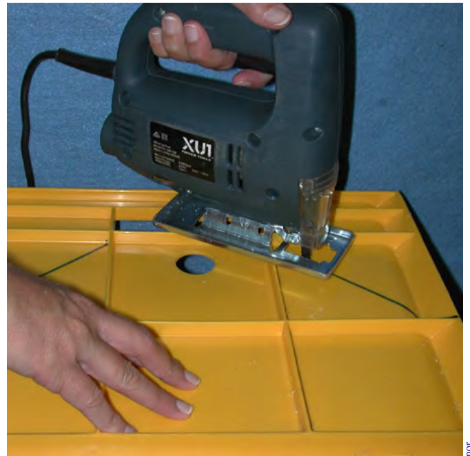
Figure 51.3 Making the biofilter container
