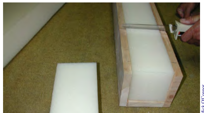
Figure 55.2 Part A Cutting the sponge into blocks
