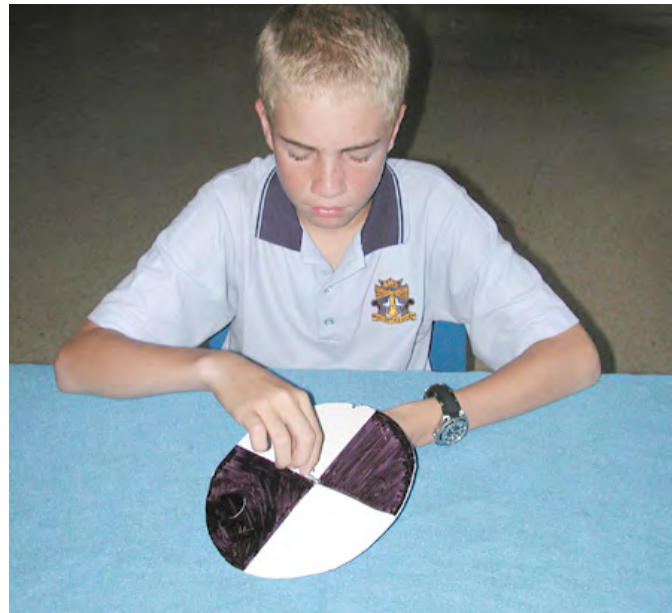
Figure 34.1 Screwing the cup hook into through the disc into the lead weights
