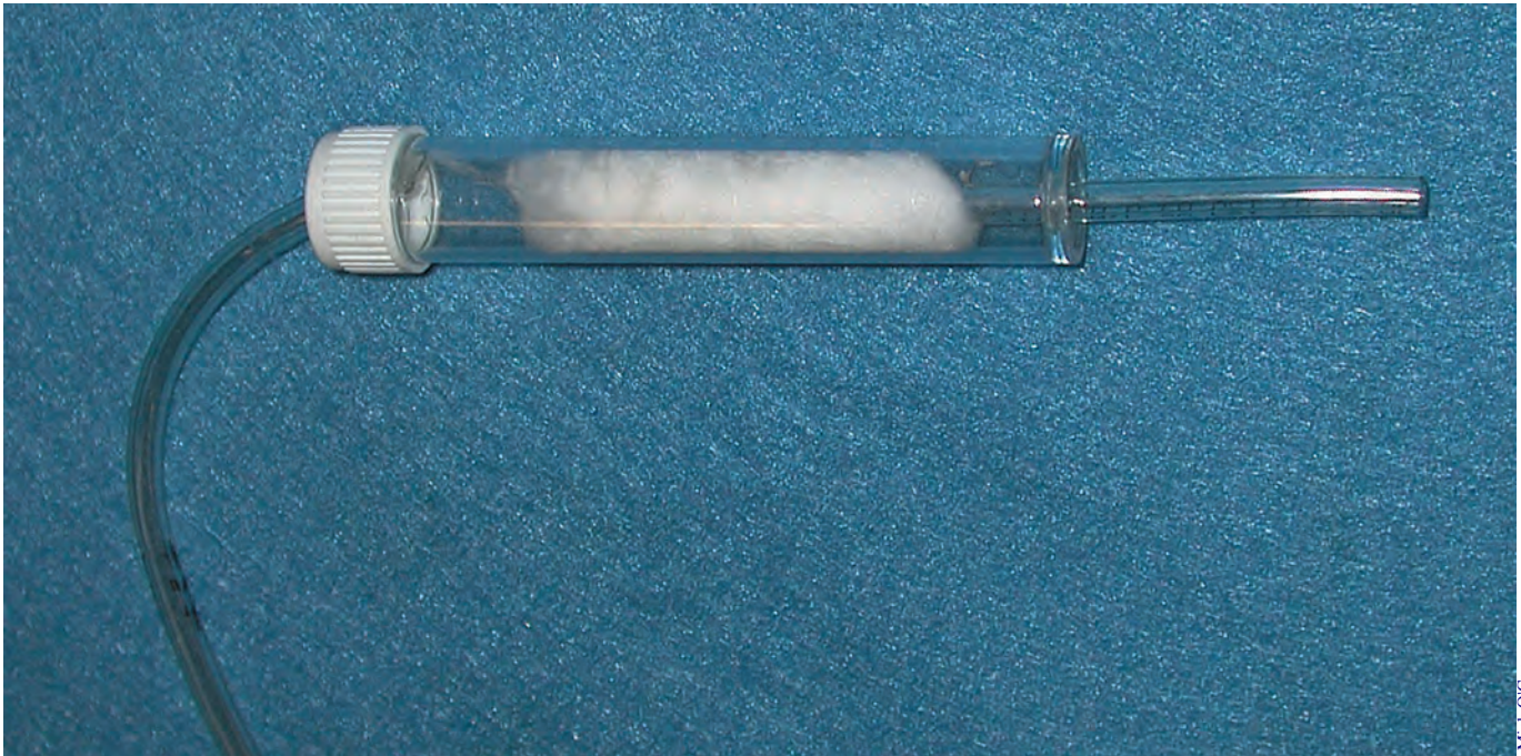
Figure 8.1 Completed air filter
