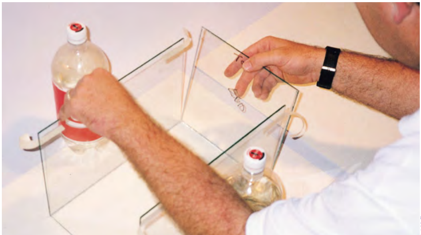
Figure 16.3 Tape the end pieces in position
