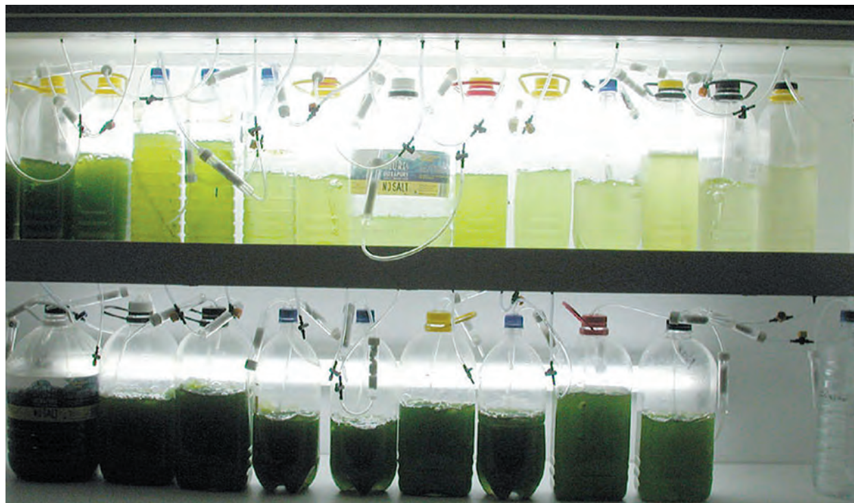
Figure 86.3 Producing algae in the light cabinet
