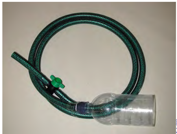
Figure 66.3 Finished syphon Mick O'Connor
