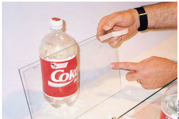
Figure 16.2 Place four pieces of masking tape at the edges you will be gluing, ready to hold the ends when finished
