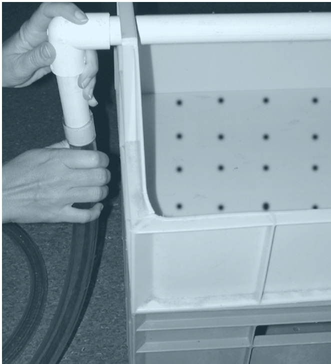
Figure 52.2 Connecting the delivery pipe
