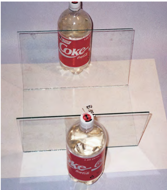
Figure 15.2 Carefully move the glued section towards the edge of the base so that it just touches the base's edge
