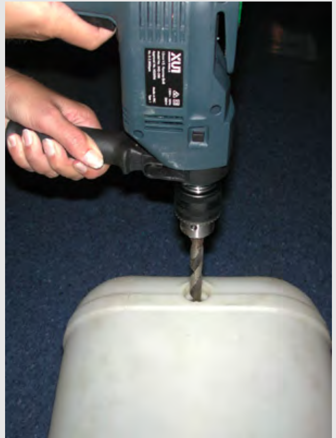
Drilling hole for standpipe
